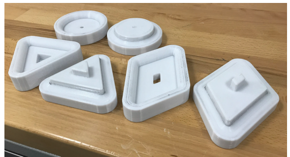
Figure 2-4: Custom flare tooling printed using polycarbonate.
